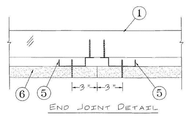
1. **Structural Steel Members\*** — Pre-fabricated light gauge steel truss system consisting of cold-formed, galv steel chord and web sections. Trusses fabricated in various sizes, depths and from various steel thickness. Trusses spaced a max of 24 or 48 in. OC, See Item 3.
