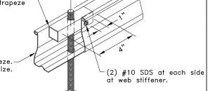
Sprinkler pipe trapeze. See hanger parts table for size.
