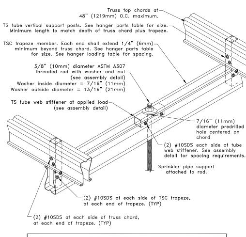
Note: Hanger rod shall be installed at a minimum of 4in. (102mm) from inside edge of truss bottom chord for TSC2.75 chords and a minimum of 6in. (152mm) for TSC3.00 or TSC4.00 chords.
